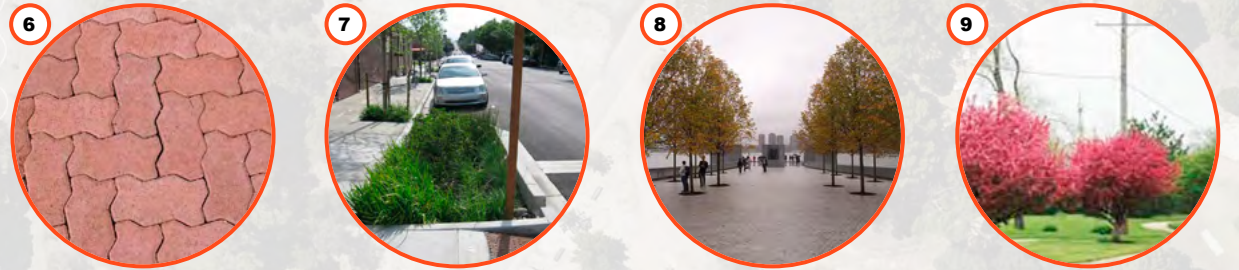
6 High contrast paving at the intersection to help define pedestrian connections/laneways, slow traffic + reinforce identity of street 7 Build-outs with slotted kerbs to maximise passive irrigation opportunities 8 New memorial plaza (optional) 9 Powerline-friendly trees to be planted under the existing powerlines
