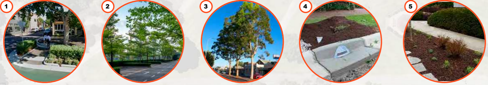
1 Formalised pedestrian crossing with pram ramps and median refuge 2 90 degree car park with avenue planted build-outs 3 Large trees with up to 10m canopies in median (optional) 4 Inlets + leaky well systems in the kerb and verge to maximise tree health and reduce flooding 5 Gravel removed and replaced with organic mulch or similar softscape to promote and improve tree health
