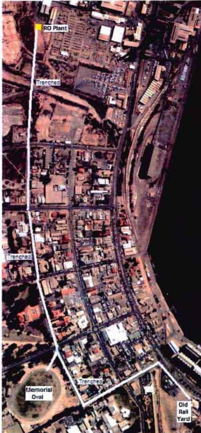
Figure F-4: Proposed pipeline route from the RO plant to the Port Pirie Township
