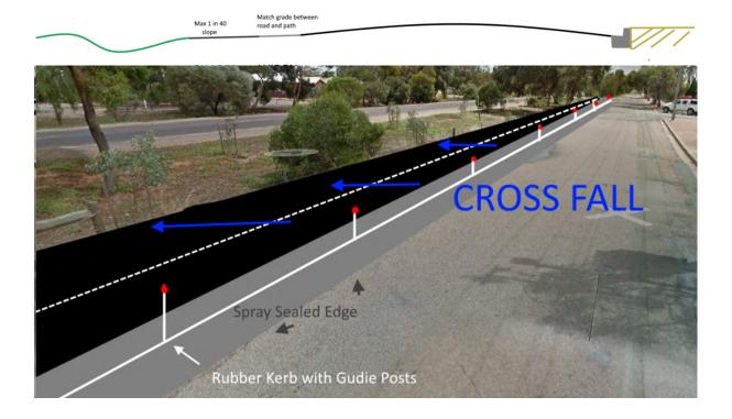
A semi mountable white rubber kerb, 230 mm wide by 125 mm high will be installed along the spray seal shoulder. The purpose of this is to prevent cars from parking on the shared pathway.
