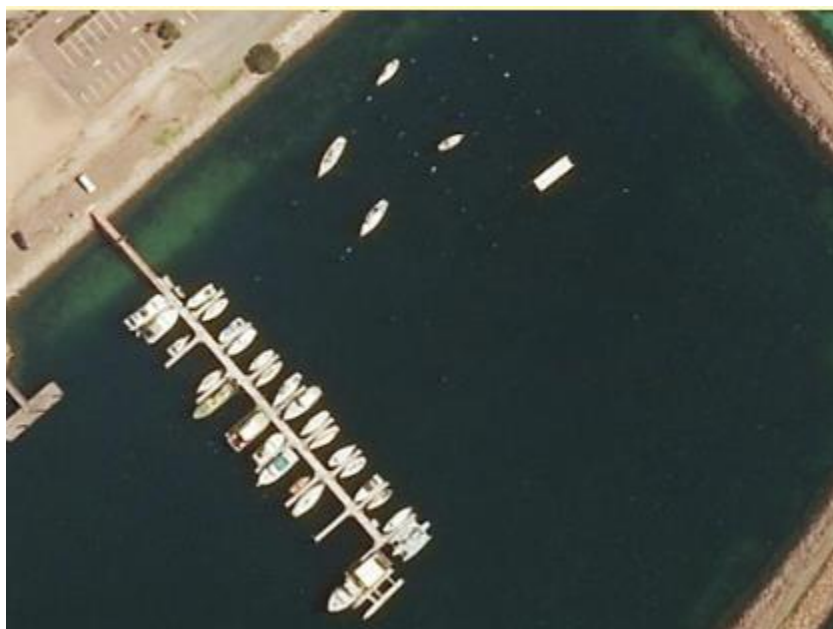
Figure 4: Whyalla Marina, note double berths and provision for larger vessels at end of finger
